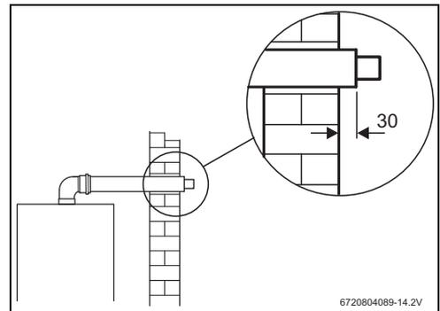
Fig. 23 Dimensioni (in mm)
