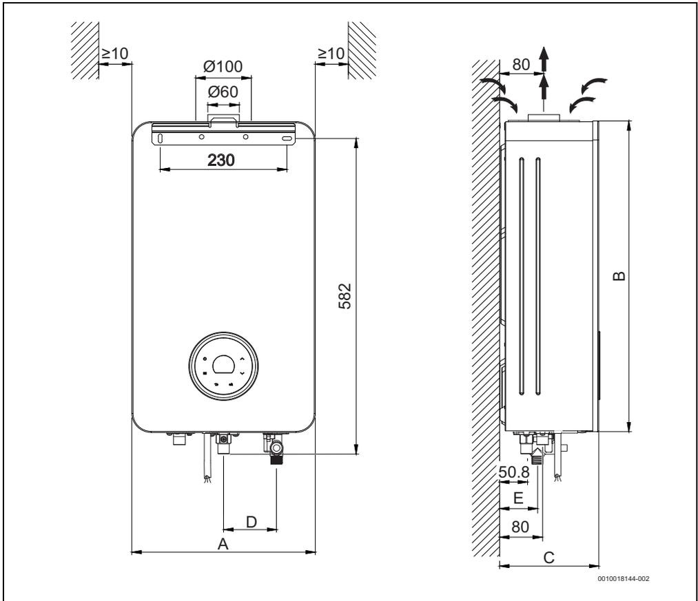
Fig. 1 Dimensioni (in mm)
